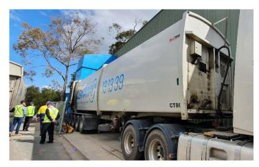
As part of assessing the future replacement of our ageing silo waste transport system, we visited Mandurah Transfer station (operated by Cleanaway) and with a throughput similar to our licenced capacity, to view their moving floor and ejector blade waste transport system in action. The image shows one of their trucks being loaded with around 26 tonnes waste to be efficiently transported to a treatment facility.
